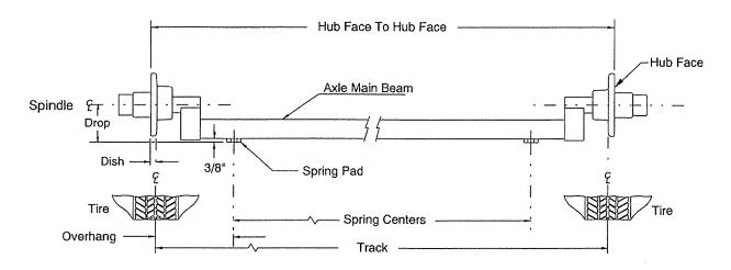
HUB FACE......is the distance from outside of hub mounting flange to outside of hub mounting flange, measured one-half way between top and bottom of hub.
